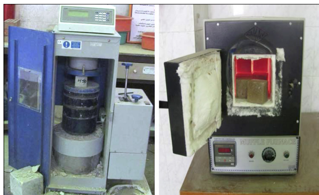
Fig. 1 Compressive strength testing machine (ADR 2000 KN) and Muffle furnace with heating rate 5°C/min.
